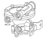
9125-5 Plug Unit Assembly 912-5 Repair Kit
